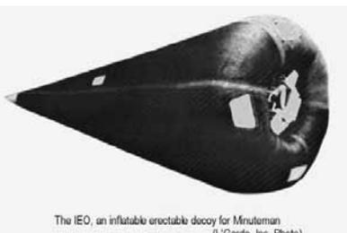
The IEO, an inflatable erectable decoy for Minuteman
