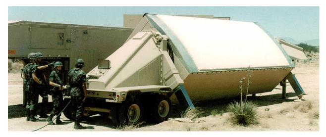
1000 km Range – Dwell Time =0.05 sec; Radar Cross Section = 0.01 m², S/N = 20, Area Searched at Distance = 4.3 km x 10.3 km 1500 km Range – Dwell Time =0.25 sec; Radar Cross Section = 0.01 m², S/N = 20, Area Searched at Distance = 6.5 km x 15.5 km
