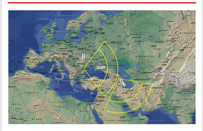
Practical Ranges at Which the FBX Radar can Acquire and Track a 0.01 m<sup>2</sup> Cone-Shaped Warhead
