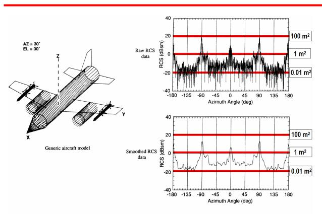
Computed raw and smoothed RCS data for generic aircraft model at 10 GHz. Smoothed data is the median within each 5° window with 2° slide.
